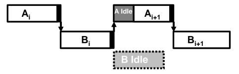
Serial Execution with No Stalls (no Hyperthreading)
